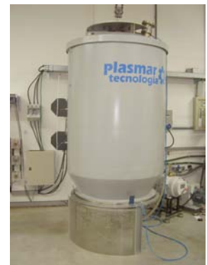
Industrial plasma nitriding furnace at a spin-off company
