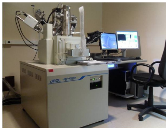
Jeol JIB-4500 combined scanning electron microscope and focused ion beam instrument equipped with nanomanipulator and X-ray microanalysis (EDS)
