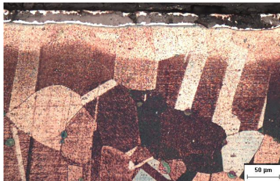
Figure 2 – Micrographs of samples treated under a pressure of 250 Pa at temperatures of 723 K during 5 hours placed at different radial positions 30 mm (a), 40 mm (b), 40 mm (c), 20 mm (d) e center (e).
