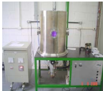
PECVD System at Clorovale Diamante
