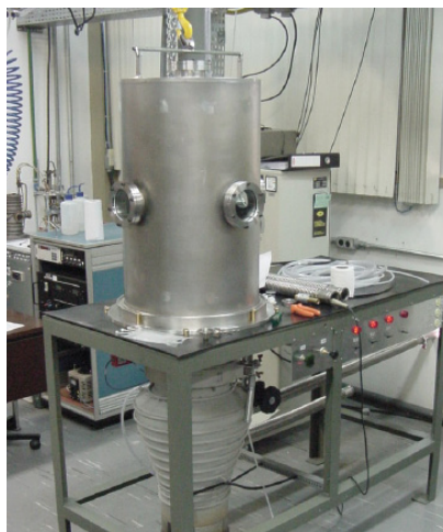
PECVD System at INPE for DLC Growth
