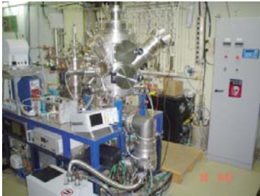
Facilities for the development of amorphous thin films using: Filtered Cathodic Vacuum Arc (FCVA), Plasma Enhanced Chemical Vapor Deposition (PECVD), ion gun, electron-beam
