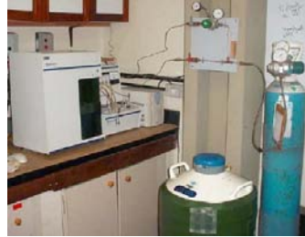
nitrogen adsorption (BET method)
