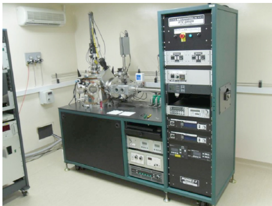
Jeol JIB-4500 combined scanning electron microscope and focused ion beam instrument equipped with nanomanipulator and X-ray microanalysis (EDS)
